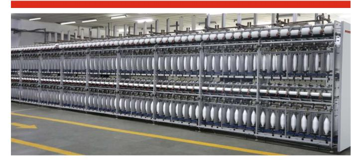
Weavetech's L-series Filament TFO Twister is for the most economic production for Low Twist Filament yarn for use in warp yarns for weaving clothing, garment, Industrial & Technical Fabrics offering high-speeds operations.
